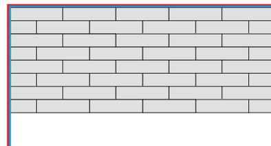
If the length of your room is a multiple of the length of the Harlequin Flexity Plus panels, cut a new panel in half and start the next row with a half-panel. It is a brickwork installation.
