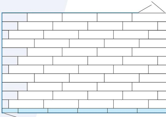
If the cut off panel is less than 300mm long use a new full panel to start the next row.
