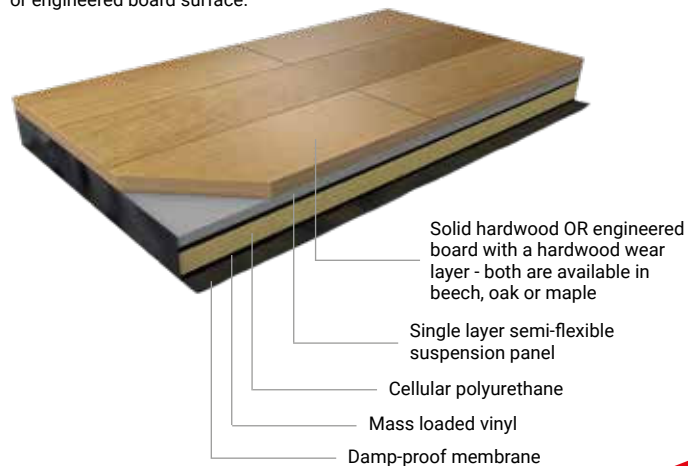
Harlequin Activity sprung floor with solid hardwood or engineered board surface.
